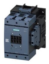
power contactor, AC-3e/AC-3 115 A, 55 kW / 400 V, AC (50-60 Hz) / DC Uc: 220-240 V 3-pole, auxiliary contacts 2 NO + 2 NC drive: conventional main circuit: box terminal control and auxiliary circuit: screw terminal
